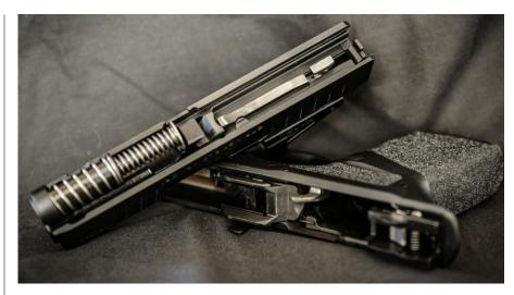
but there is no grip safety on this pistol. The firearm has a non-proprietary front rail that allows the installation of all common lights and laser if desired. Along with being the highest capacity micro-compact with a three-inch hammer forged barrel, it measures a mere one inch in width and weighs just 18.3 ounces empty. With the flush-
